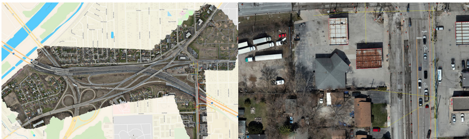
The project orthomosaic, captured with a Matrice 350RTK, was processed in PIX4Dmatic and imported to PIX4Dcloud to overlay design files. Zooming up on the orthomosaic in PIX4Dcloud shows the high resolution and detail of the map; the lines represent DXF files of reworked utilities
