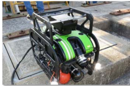
Multi-Sensor Inspection (wet pipe)
