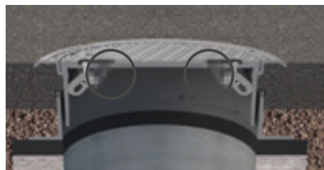
The SELFLEVEL® access assembly requires two VERSACAM security locks and security bolts.
