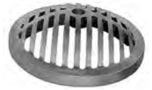
Type O1 Beehive Grate Approx. 135 sq. in. open area 4" height above frame
