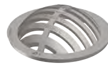
Type O1 Beehive Grate Approx. 140 sq. in. open area 5 1/4" height above frame "DUMP NO WASTE!" lettering and trout image
