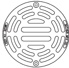
Type M1 Grate Approx. 107 sq. in. open area
