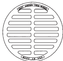
Type M Grate Approx. 185 sq. in. open area
