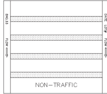
V-4823-3 Vane Grate Approx. 650 sq. in. open area
