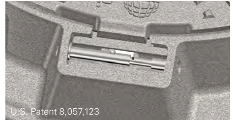
Option 2—Retrofit (cutaway view shown) The retrofitting captive hinge pin can be installed anytime if a preinstalled pin hasn't been used. The pin comes with a spring built within the pin, which sets during installation to permanently secure the hinge to the frame.
