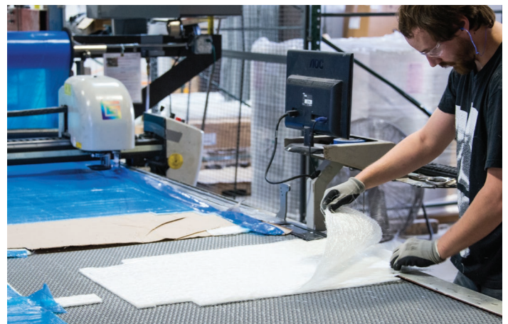
Engineered fiberglass fabric being cut on material cutter.
