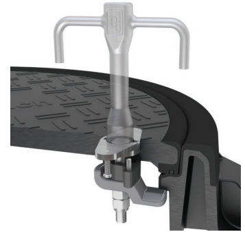
The special key is used to turn the lock and engage the paddle with the frame. In this locked position, the key can then be removed.
