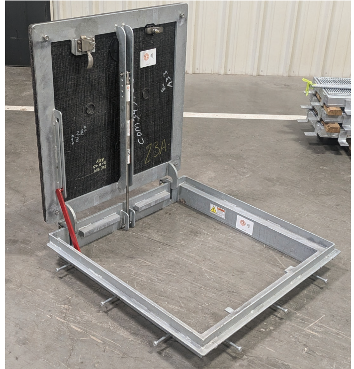
This example shows a custom fabricated steel access hatch combined with the advantages of a composite cover, making it ergonomic, non-corrosive, and non-conductive while maintaining a heavy duty rating.
