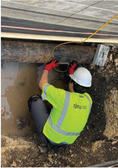
Broadband electromagnetic (BEM) inspection can determine relative pipe wall thickness.
